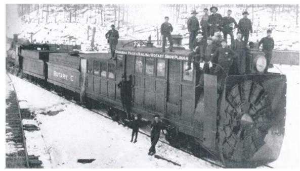
Jull obtained Canadian and American patents for his design and in 1884 the Leslie Brothers assembled the prototype on a C.P.R. flatcar. The winter of 1884 was over before the unit could be tested, but CPR obliged by filling a rail cut at
